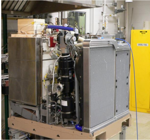
Figure 6. Gen4 System Photo with Test Instrumentation in Place. Shown from Left Front to Show Air System (black cylinders) and Fuel Supply System (immediately behind air system)
